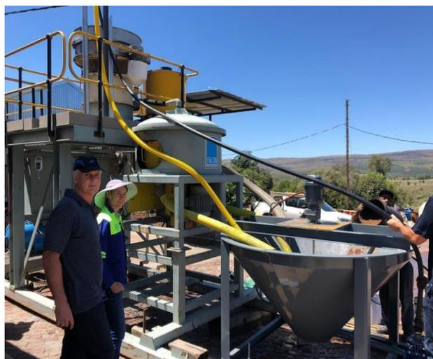
Milling of Zanaga material in test facility
